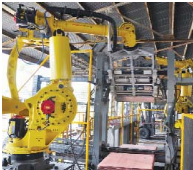
Xstrata Technology's new robotic stripping technology which has been designed for use in the copper refining industry.
